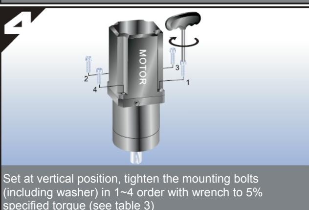
Set at vertical position, tighten the mounting bolts (including washer) in 1~4 order with wrench to 5% specified torque (see table 3)
