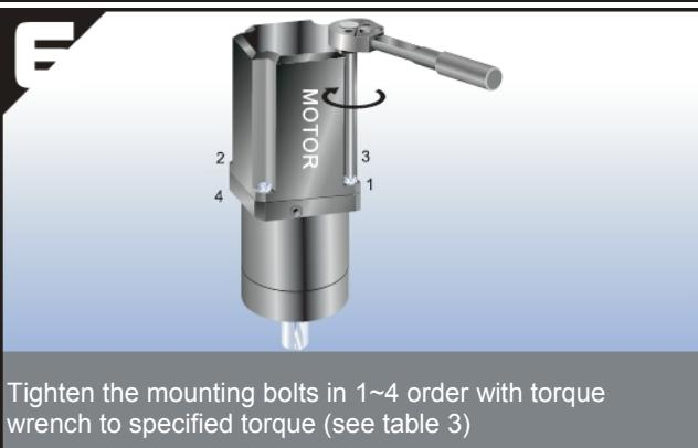
Tighten the mounting bolts in 1~4 order with torque wrench to specified torque (see table 3)
