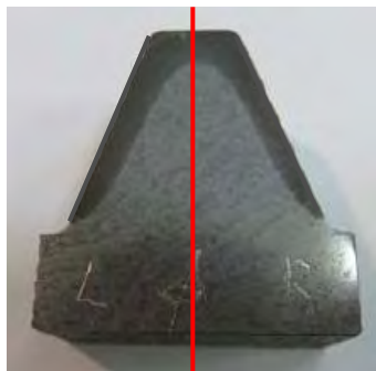
Qualified induction hardening and teeth grinding
